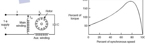
Fig. .1.6. Permanent split capacitor motor (=) Connection (>) Torque-speed characteristiS
