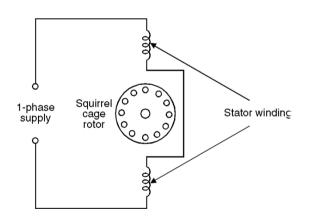
Fig .1 Elementary single phase induction motor.
