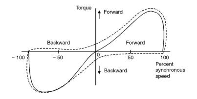
Fig. 1.3. Torque-speed characteristic of a 1-phase induction motor taking into account changes in the flux waves.
