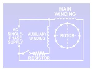
Figure. Resistance-start ac induction motor.
