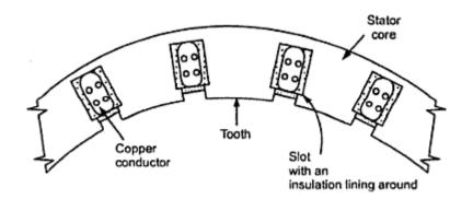
The armature core is supported by the stator frame and is built up of laminations of special magnetic iron or steel iron alloy the core is laminated to minimize the loss due to
