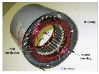
Figure. Single phase stator with windings.
