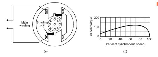
Fig. .1.8. Shaded-pole motor and typical torque-speed characteristic.
