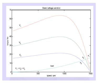
Figure. Speed-torque curves: voltage variation
