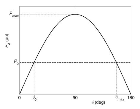
Fig 5.2 A typical power-angle curve
