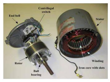
Figure. Induction motor components.
