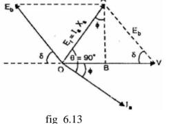
$AB = E_r \cos \phi = I_a X_s \cos \phi$  $AB = E_b \sin \delta$  $E_b \sin \delta = I_a X_s \cos \phi$  $I_a \cos \phi = \frac{E_b \sin \delta}{X_s}$
