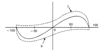
Fig. 1..2. Torque-speed characteristic of a 1-phase induction motor based on constant forward and backward flux waves
