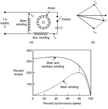
Fig. 1.5. Capacitor start motor (=) Connection (>) Phasor diagram at start (?) Speed torque curve.
