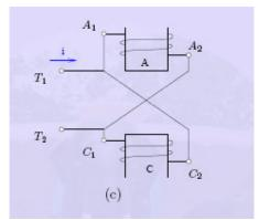
Figure: Pole Changing: Various connections
