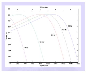
Figure. Torque-speed curves with E/f held constant
