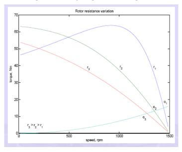
Figure. Speed-torque curves: rotor resistance variation
