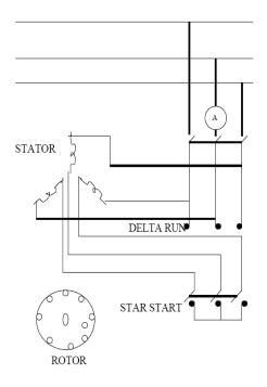
For starting, the stator windings are connected in star and when the machine is running the switch is thrown quickly to the running position, thus connecting the motor in delta for normal operation. The phase voltages & the phase currents of the motor in star connection are reduced to  $1/\sqrt{3}$  of the direct -on -line values in delta. The line current is 1/3 of the value in delta.
