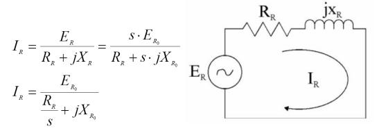
The rotor circuit can be represented as
