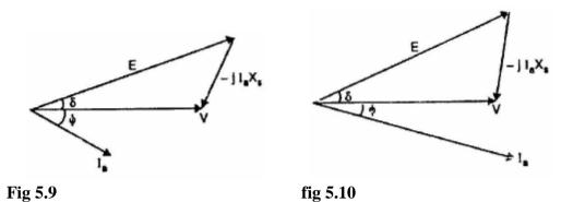
Increasing the mechanical input power to the prime mover will notchange the speed ultimately but will increase the power angle d. As a result, the change of driving torque controls the output kW and not the kVAR. When this change takes place, the power factor of the machine is practically not affected
