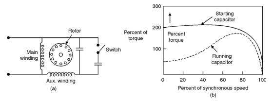
Fig. 1.7. (=) Capacitor start capacitor run motor (>) Torque-speed characteristic.
