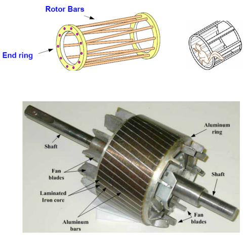
Figure. Squirrel cage rotor
