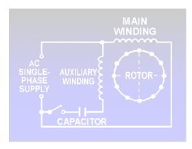
Figure. Capacitor-start, ac induction motor.
